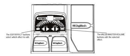
When the stored value of an effect is changed, the lower right decimal point in the display lights indicating you need to store the changes. Changing presets, or turning the power off before storing any changes will erase any changes made and revert to the stored values for the preset.
